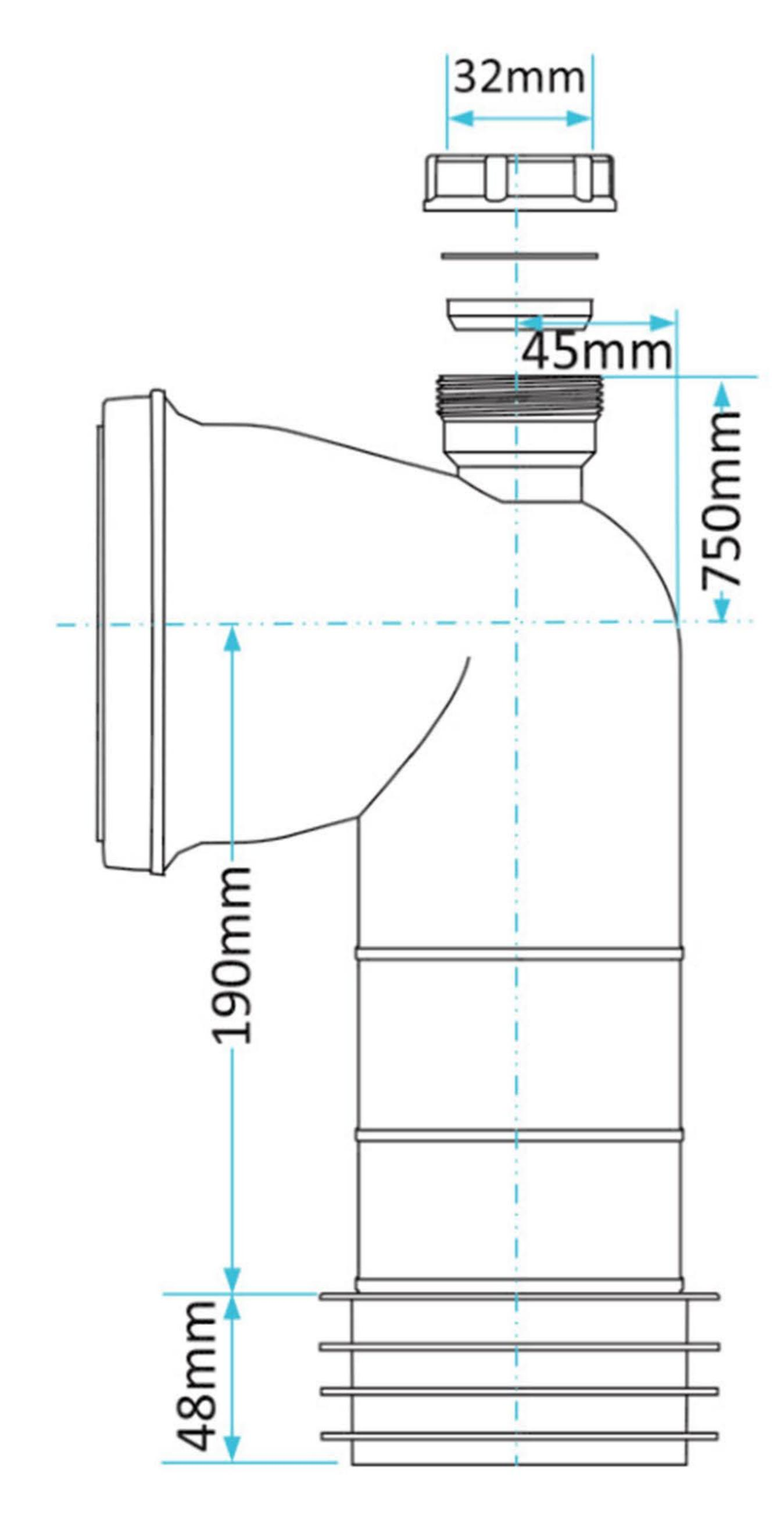
All drawings contain the necessary measurements which are subject to standard tolerances. Exact measurements, in particular for customised installation scenarios, can only be taken from the finished ceramic piece.
