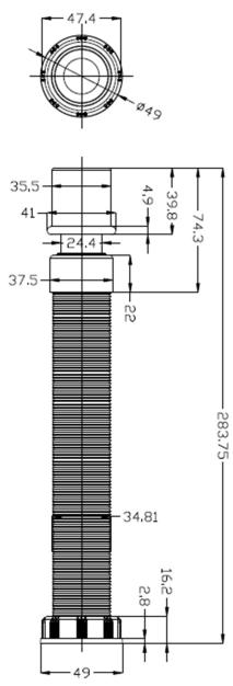
All drawings contain the necessary measurements which are subject to standard tolerances. Exact measurements, in particular for customised installation scenarios, can only be taken from the finished ceramic piece.
